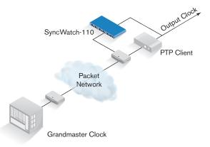
Figure 4. PTP performance testing with the SyncWatch-110
