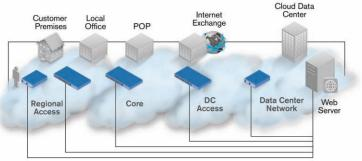
Figure 6. Testing cloud services from the carrier's network
