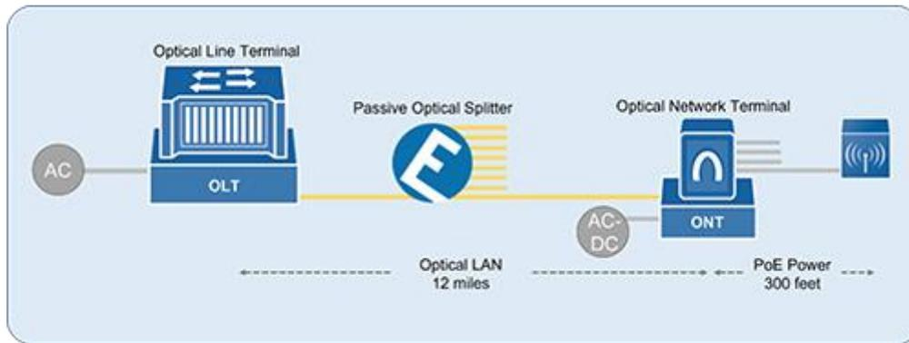
Figure 3: An Optical LAN using Class 2 power to connect an ONT out 2,000 feet
