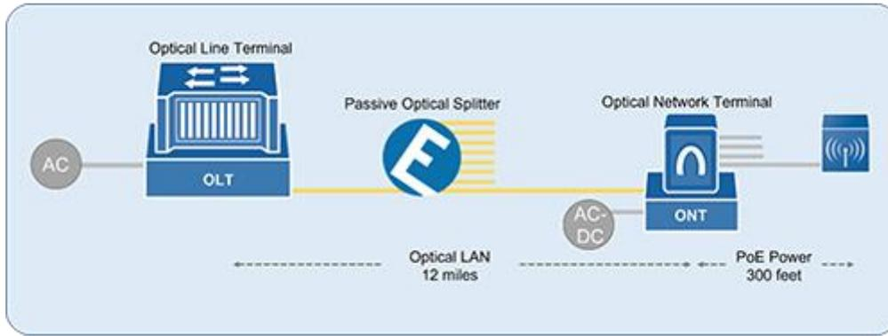
Figure 4: An Optical LAN with Class 4 reaching 6,500 feet to energize an ONT
