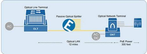
Figure 3: An Optical LAN using Class 2 power to connect an ONT out 2,000 feet
