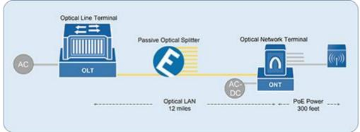
Figure 4: An Optical LAN with Class 4 reaching 6,500 feet to energize an ONT
