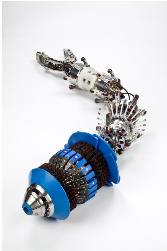
Figure 2: MFL Vehicle (Courtesy of Baker Hughes, a GE Company)
