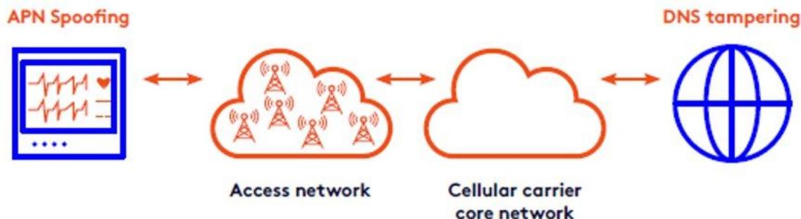
Figure 1: How a data channel rerouting attack works
