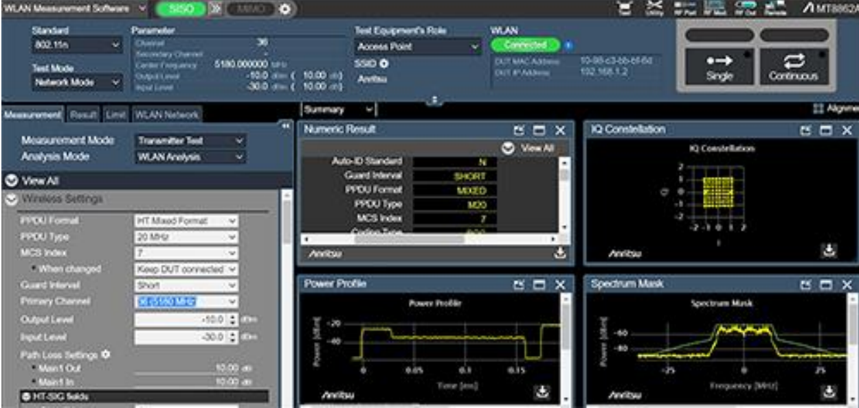
Figure 3: Instrument display showing IQ constellation, power profile, and spectrum mask of a WLAN signal click to enlarge
